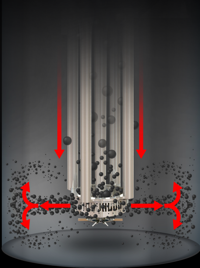
Above: Rotor stator particle flow Below: Rotor stator shearing process
