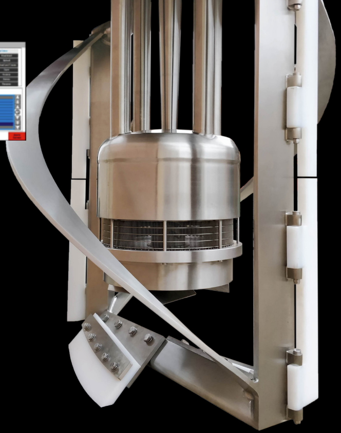
Above Right - Schold VIM with Lifting Helical Arms and Scrapers Above Left - Schold VIM HMI Screens
