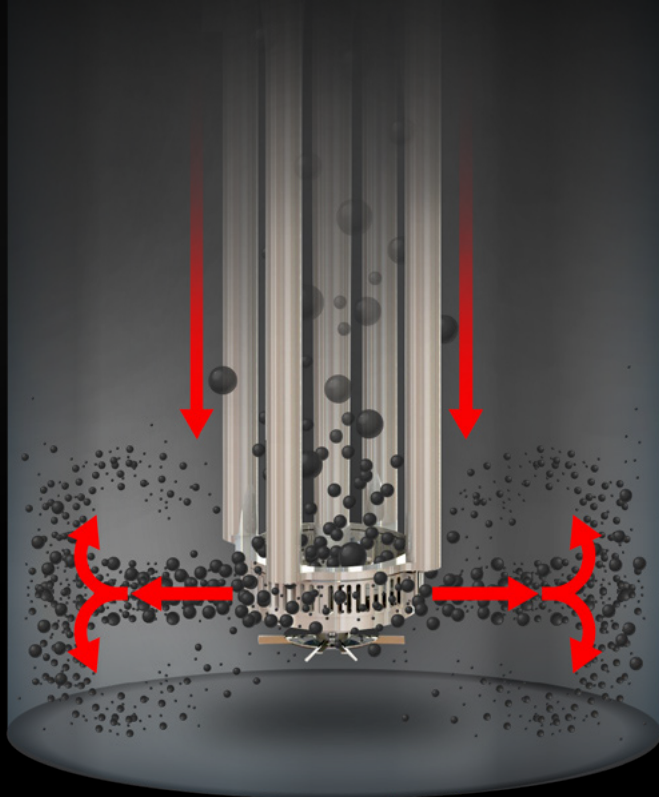
Side tank cutaway of Schold Rotor Stator and particle flow.
